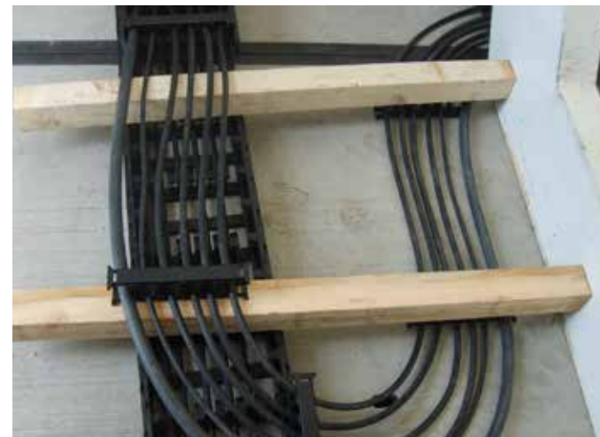
The energy chain® equipped with the test cables
