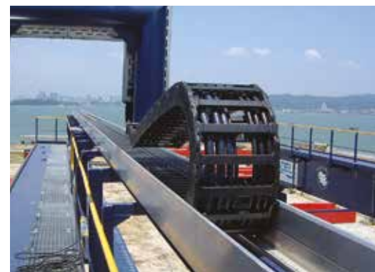
Use of an energy chain® including chainflex® cables in a port crane
